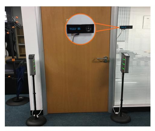
Once the pre-set threshold level is reached the units will sound an alarm and flash red at the head units to deter further entry. When the occupancy level is reduced the units will reset and clear the alarms.
